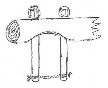
Fig. 16: Wooden staves are similar to the skeis used in many ox yokes, but with a dropped hitch point yoke, the wood must be round, not rectangular, so that it cannot injure the neck or shoulder.
