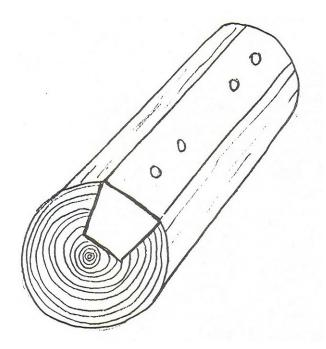
Fig. 9: Traditionally a large tree was split and one section was used to make the yoke beam. This eliminated the heartwood, and the tubular grain
