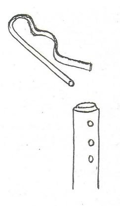
*Fig 17: A pin to hold the bow can be made from the spring of a broken bicycle seat.*
