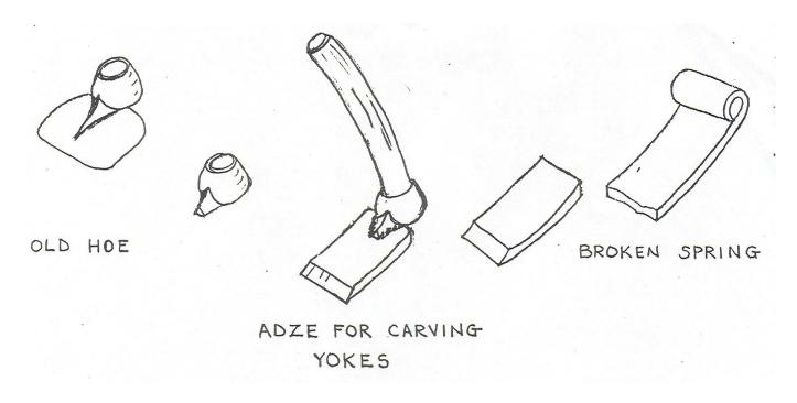
Fig. 13: A blacksmith can make an adze from an old hoe and a spring from a truck.
