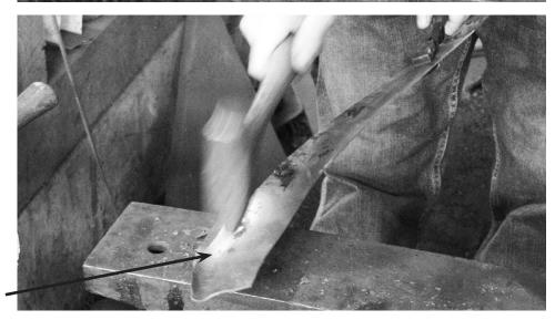
Use a straight pein to hammer the outside edge into a swedge block or groove, forming a bend along the full length of the blade.
