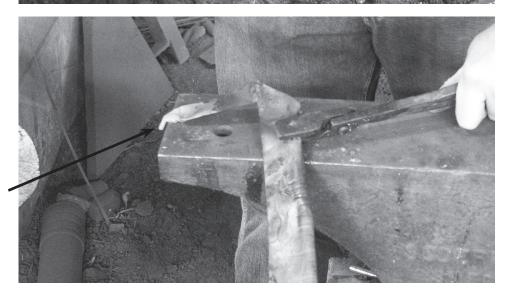
Pin, bent at 90 degrees to the flat of the rest of the blade.
