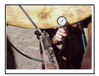
cylinder. This device allowed instantaneous measurements of draft (lbf), and when combined with time and distance, power output (hp).
