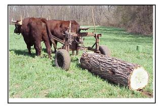
grasp the hitch end of the log for transport. Under a load the tongue weight came off the yoke as it counterbalanced the rearward torque of the log.
